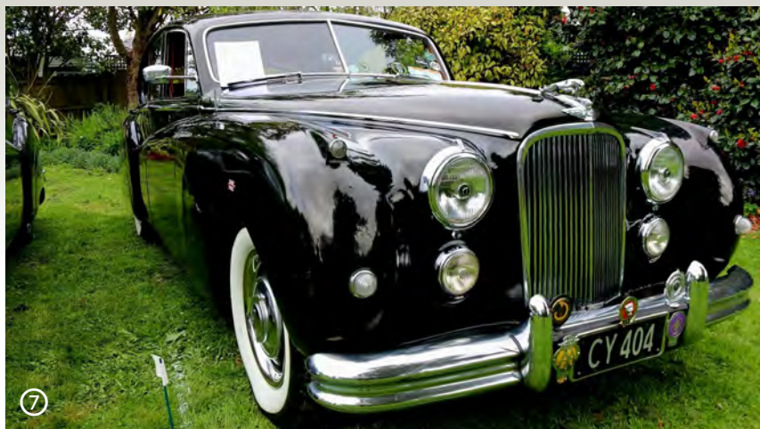
④ Probably the most outstanding and highly modified Mark VIII of Graeme & Nancy Blackstock of New Plymouth. Graeme spent years modifying the car so that Nancy, in a wheelchair, can go up a ramp into the back of the car. It is now based on an XJ6-R undercarriage and engine.
