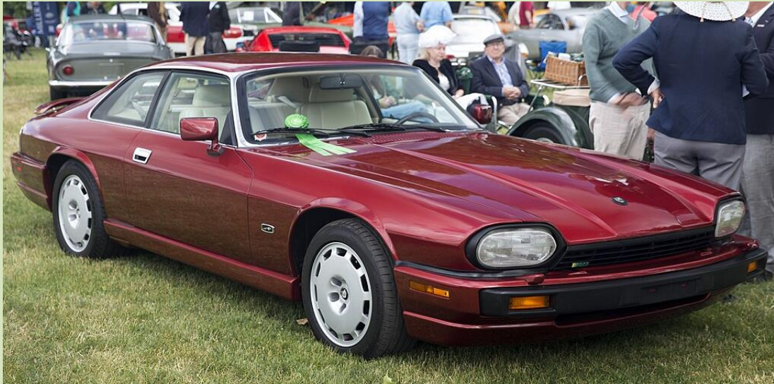
A 1994 XJRS showing the facelift with rubber bumper inserts, smaller rear buttresses, revised front lights and the removal of the rear quarter pads with larger rear windows (Internet).
