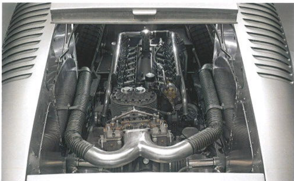
The 16-cylinder engine of the Auto Union Type 52 "Schnellsportwagen". Seriously LOUD.
