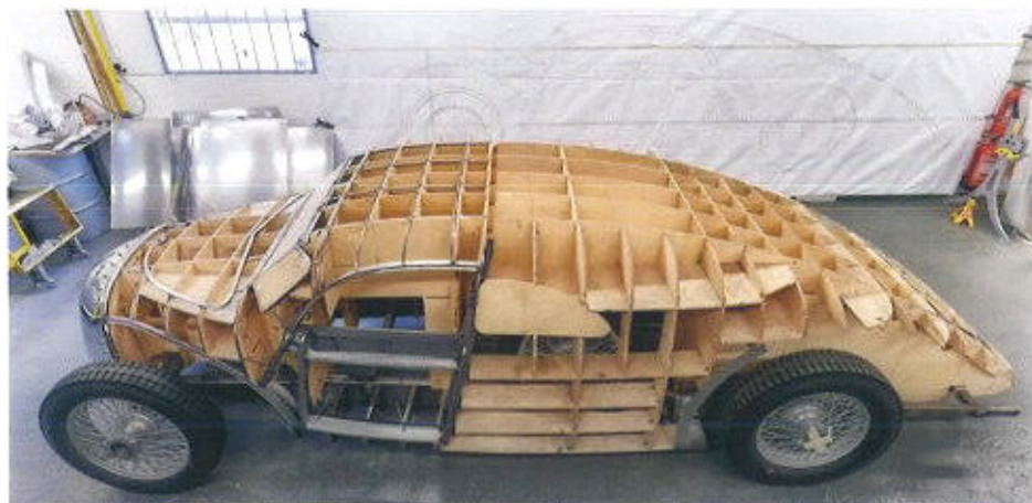
The painstakingly-created wooden buck on which the new body panels were formed. You may also be able to see the large scale outline drawing on the wall behind.
