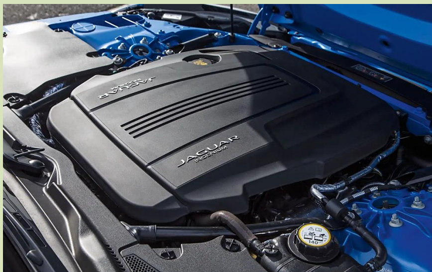
The 2 litre Ingenium motor of the 4 cylinder F-Type (Autocar).
