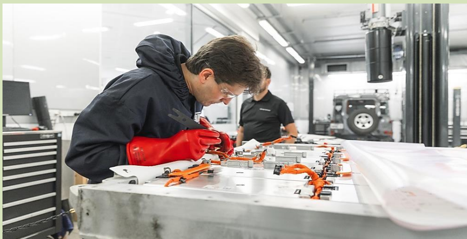
Unscrewing the faulty module from the base plate and replacing it with a new one is a delicate operation.
