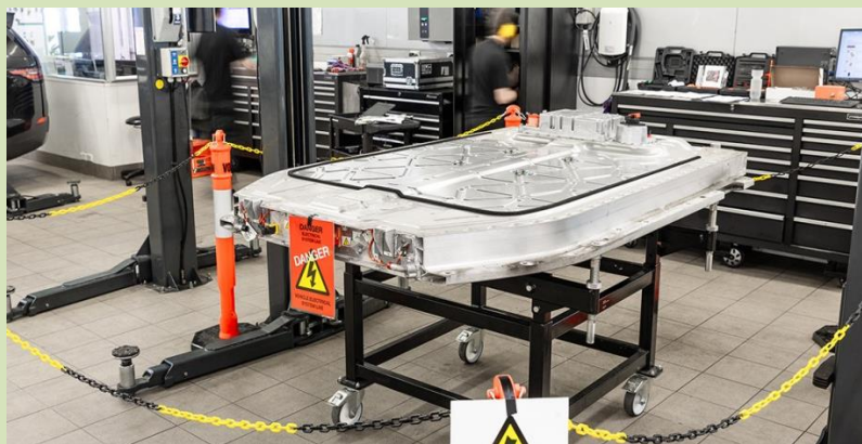
An example of the under floor I-Pace battery with the protective cover in place and the work area roped off.
