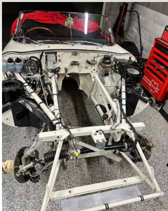
Empty engine subframe. Note front suspension dismantled to remove reaction plate for torsion bars (1)
