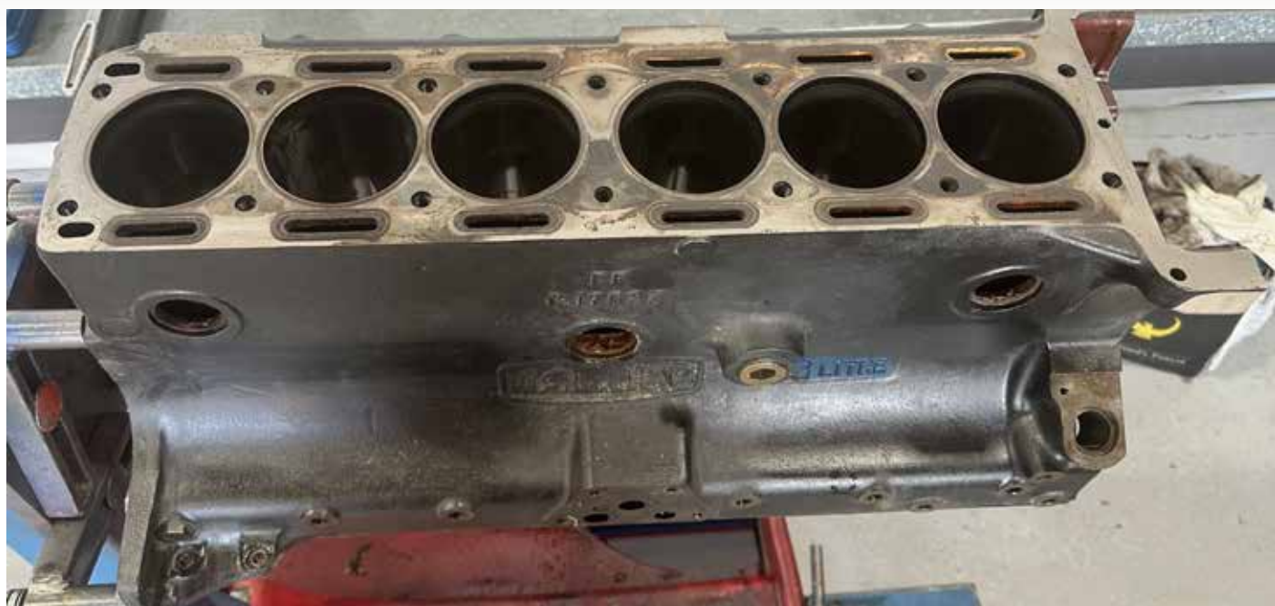
My 3.8 engine stripped down. Note how tight the space is between cylinders 1 & 2/5 & 6 (4)
