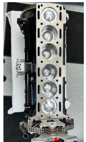
Engine upright and assembled short engine: Note drip feed oil reservoir (arrowed)
