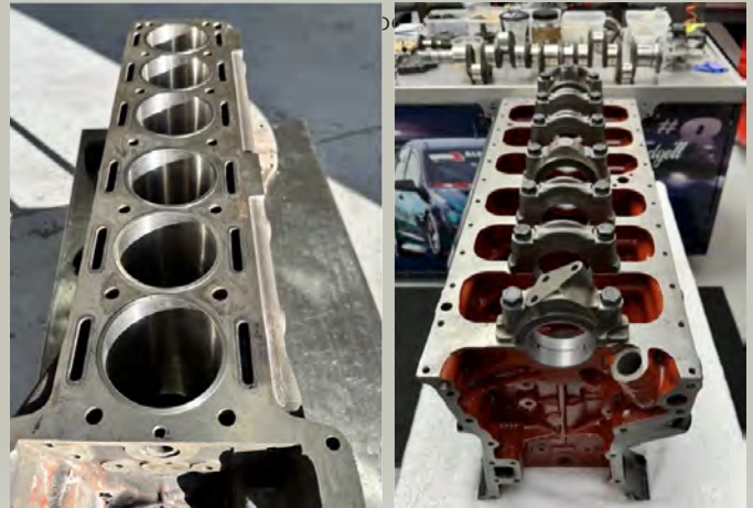
Block with new flanged liners installed and Block after liners bored and 2 pack painted internally
