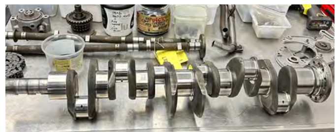
Polished Crankshaft and parts laid out at Edgells. Note turned down 75mm journal for Viton "Flexy" rear main seal
