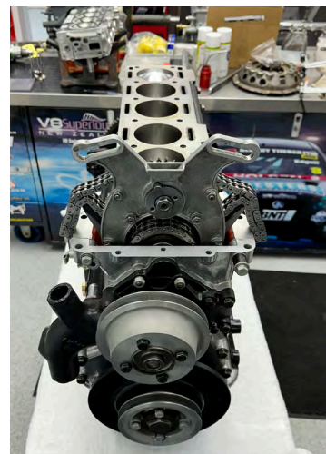
Engine upright and assembled short engine: Note drip feed oil reservoir (arrowed)
