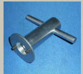
Diagram of front timing gear bracket and timing chain adjuster tool (readily available)
