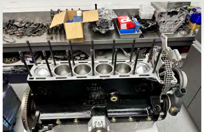
ARP hi-tensile studs installed in completed short block
