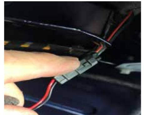
x*ix*) intermediate loom reconnected to main boot loom
