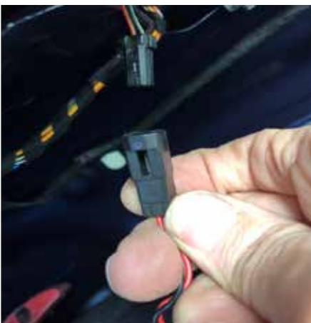
x*iv*) cable connector releasing intermediate loom
