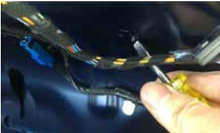
x*ii*) Pressing end of end of mushroom clip holding intermediate loom, back through boot lid inner panel
