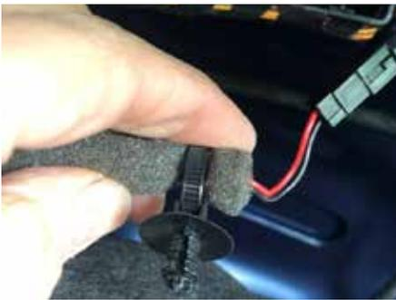
x*iii*) released mushroom clip and intermediate loom (foam wrapped). Note cable connector clip at top right of frame.
