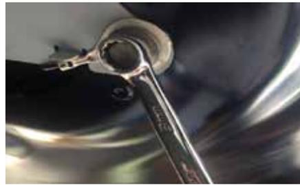
x*v*) releasing earth cable of intermediate loom
