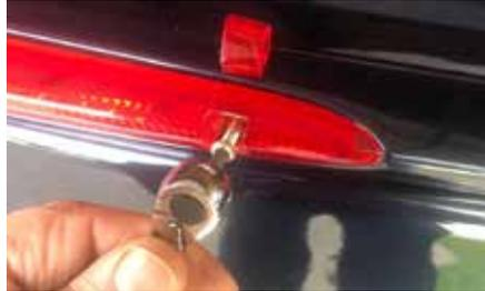
iv) removing LED unit fixing screws with torx ratchet
