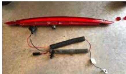
x*vii*) new LED unit connected to intermediate & earth cables.
