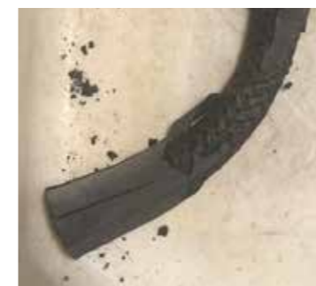
Disintegrated rubber conduit (new when installed in 2015) - Ethanol damage possibly?
