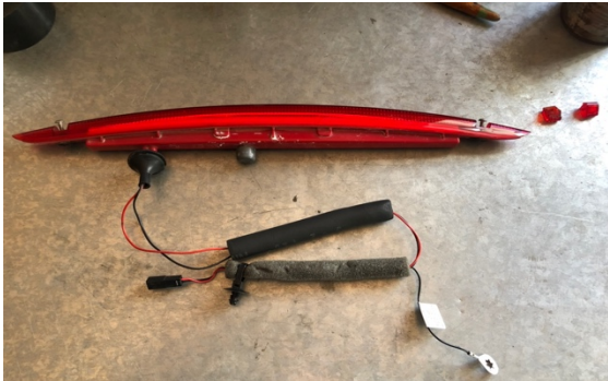
xvii) new LED unit connected to intermediate & earth cables.
