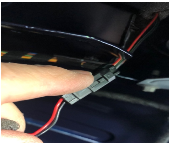
xvix) intermediate loom reconnected to main boot loom
