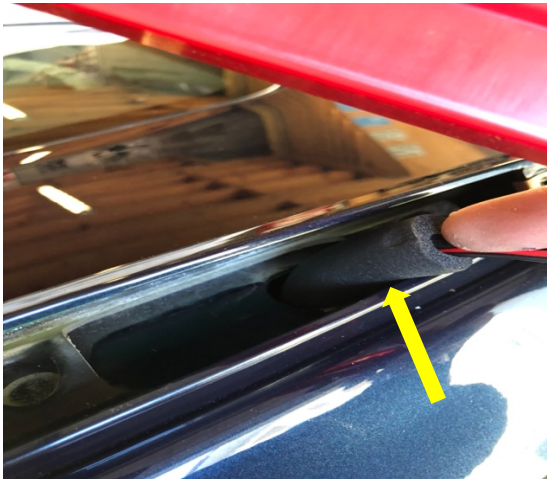
xviii) new LED cables fed back through boot spoiler
