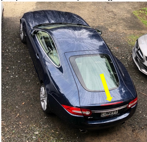
i) Failing boot spoiler mounted LED brake light.
