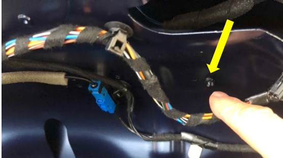
xii) end of mushroom clip holding intermediate loom
