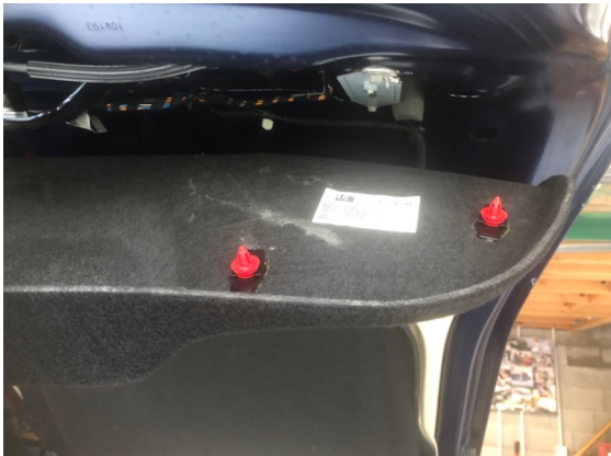
vii) Right hand side trim clips removed.
