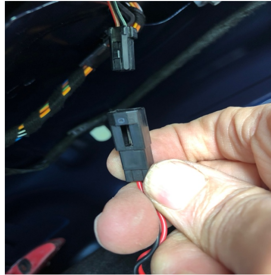
xiv) cable connector releasing intermediate loom
