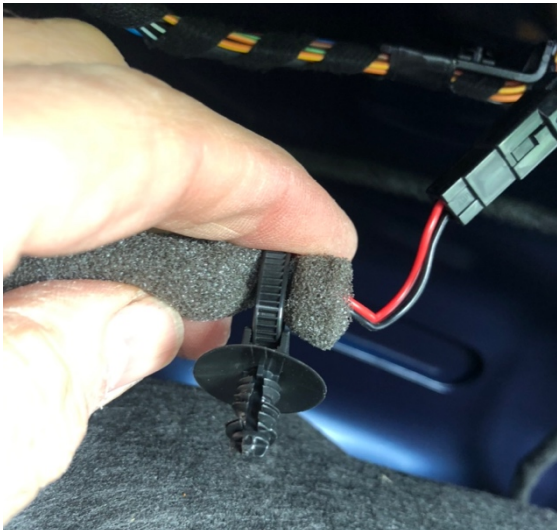
xiii) released mushroom clip and intermediate loom (foam wrapped). Note cable connector clip at top right of frame.
