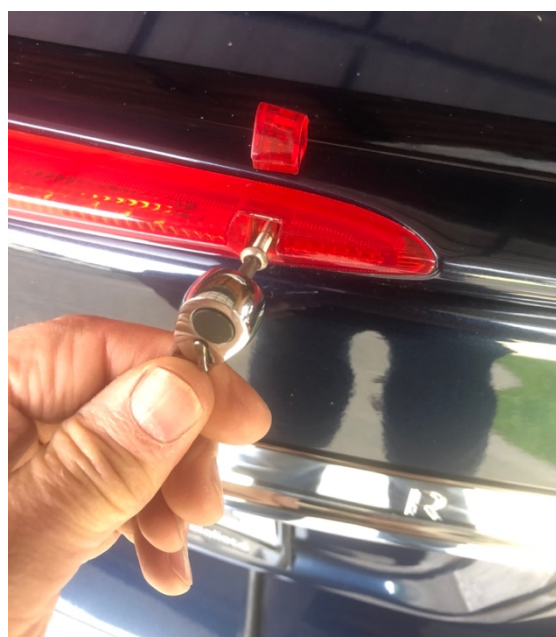
iv) removing LED unit fixing screws with torx ratchet
