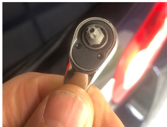
iii) Two Torx/star head screws easily removed with the correct screw bit.
