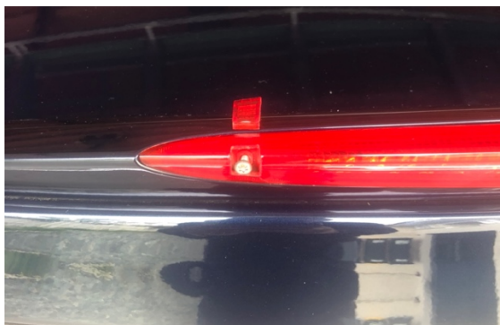
ii) Easily removed cover clip over torx screw.
