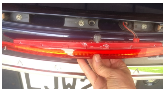
v) That went well and the lamp unit released after a gentle pull. Note the red and black cables
