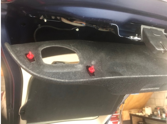
vi) Left hand side trim clips removed.
