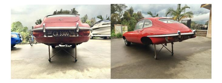
Next the IRS assembly was removed with a floor jack
