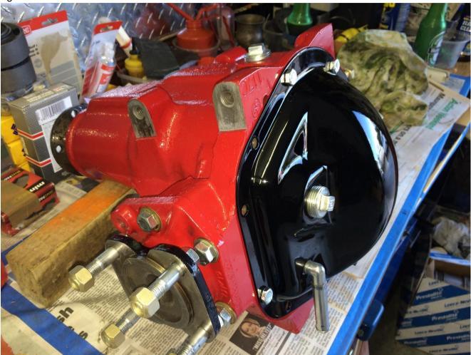
Next the two output shafts with new bearings could be fitted to the diff head followed by two new brake rotors and the rebuilt brake callipers. This was then mounted back into the main crossmember.
