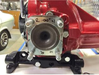
Four new universal bearing cap sets were fitted to both half shafts, then bolted to the rotor flange with the corresponding number of newly plated shims for adjusting the rear wheel camber.
