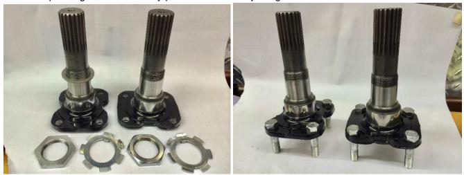
With all the painting complete the rear axle hubs could be rebuilt. These were exceptionally complex trying to achieve the correct end float between the two tapered bearings, but I eventually got there.
