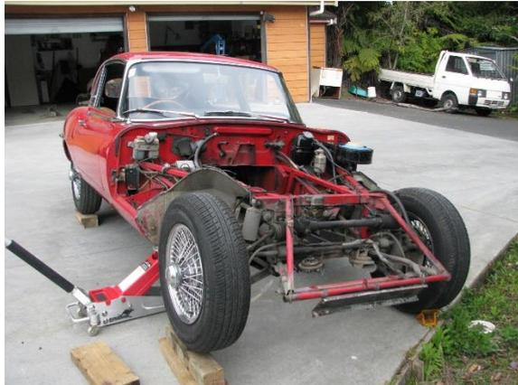
Then the body was back in the garage where every single component from the firewall forward was removed, cleaned and prepared for painting, polishing or plating. Bright zinc was the plating of choice.
