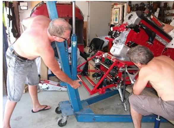
Now all the engine components could be fitted including radiator, heater box, hydraulic cylinders and all the pipes and hoses.
