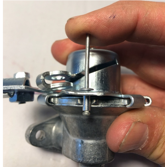
8) pop rivet inserted into aligned hole through outer casing and two small projections on alloy valve body.
