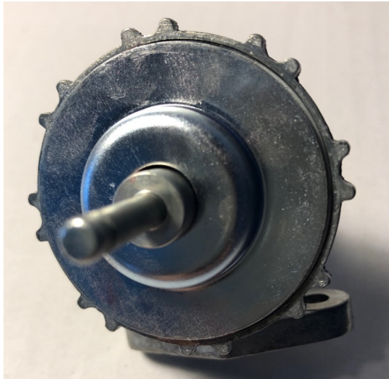
5) Zinc plated disc e) that sits over the spindle c) and diaphragm d) on valve body a).
