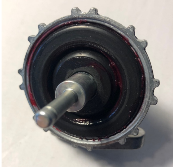
4) New rubber diaphragm (d) inserted into new alloy valve body a). Note liberally applied rubber grease.
