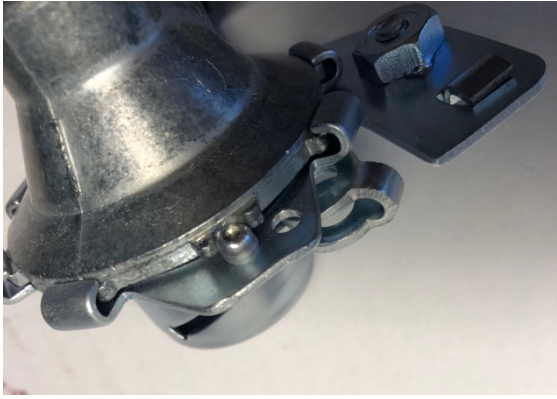
10) installed pop rivet
