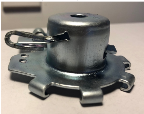
6) Zinc plated activation lever inserted into outer casing
