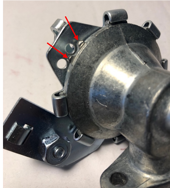
7) Re-plated outer housing b) installed onto new alloy valve body, with pop rivet holes aligned.
