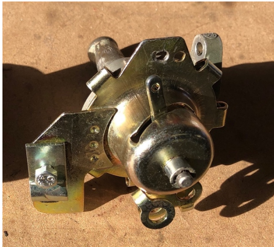
1) Passivated zinc replacement valve; also no part No.
