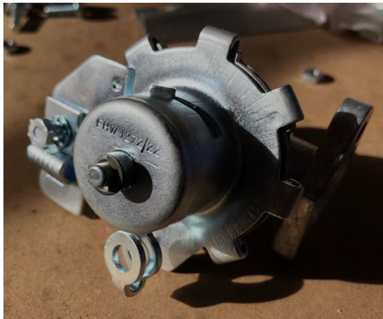
2) Original valve: zinc plated & Part No. FHW 1272/22
